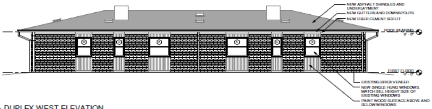
DUPLEX WEST ELEVATION 1/4" = 1'-0"
