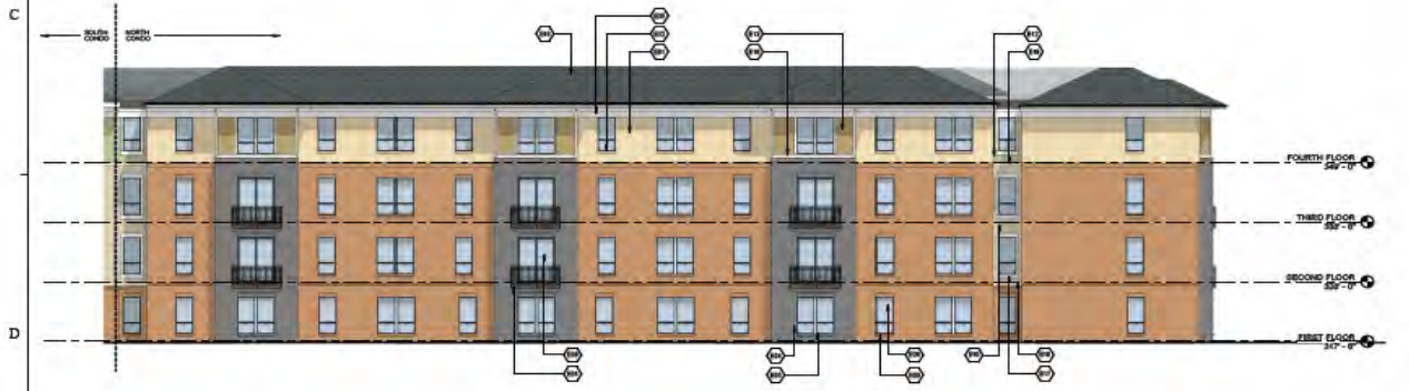
1 ENLARGED ELEVATIONS - NORTH CONDO - EAST FACE SCALE: 1/8" = 1'-0"
