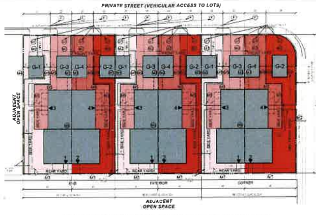
SPEX DETAIL: QUADRUPLEX TYPICAL LOT LAYOUT (ADJACENT OPEN SPACE AT REAR) SCALE 1" = 32'
