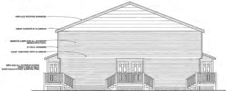
2 BUILDING ONE & THREE - TYPICAL SIDE ELEVATION SCALE: 1/8" = 1'-0"
